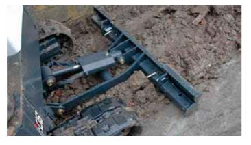
Equipped with expandable undercarriage and blade as standard. There is no need to remove and reinstall the blade extensions.
