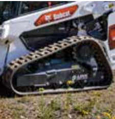
Torsion Suspension – 5 Link System
