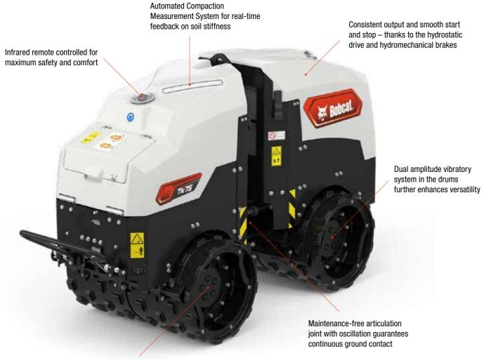
TR75 is available with optional drum extensions, making the machine extremely versatile
