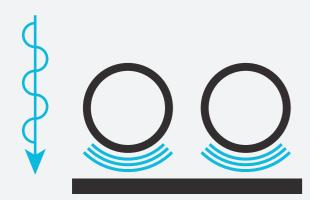
0.3 mm amplitude for asphalt applications
