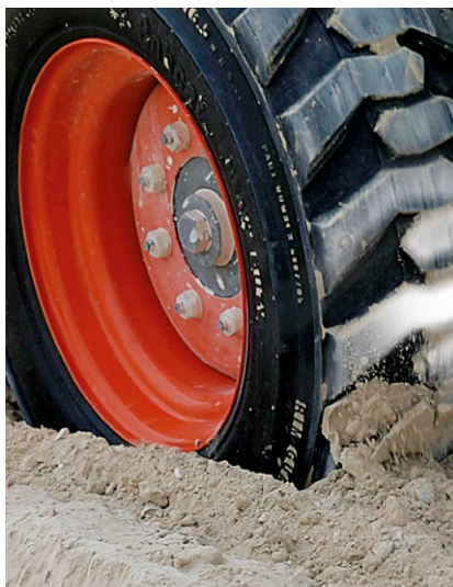
CUVED LUGS IMPROVING TIRE CLEANOUT
