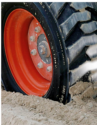
CUVED LUGS IMPROVING TIRE CLEANOUT
