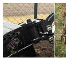
Mechanical German type coupler (MS01) Digging bucket with tilt function
